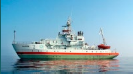
MARANDA, 165 kW FC Operation 2019 Finland
